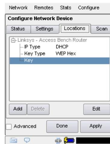
7. If the connection requires a password, select the **Key** parameter and press the **Edit** button near the bottom of the screen.
